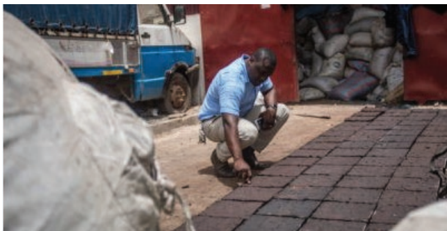
An engineer inspects paving blocks made from recycled plastics in a suburb of Accra, Ghana
